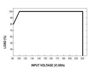
\* De-rating is needed under low input voltage.
